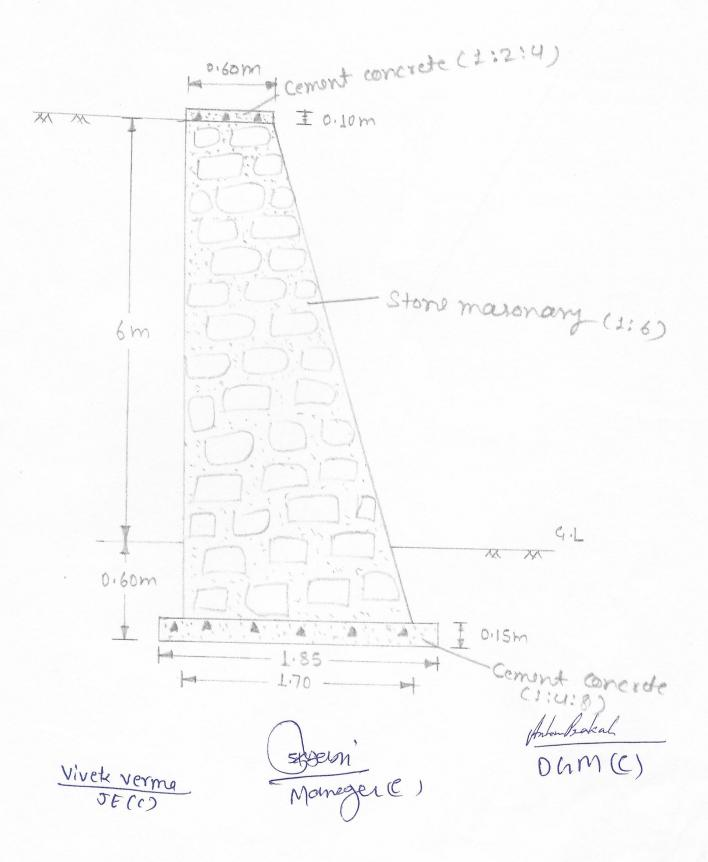
Cross-section of wall A (For 39 M WALL)
